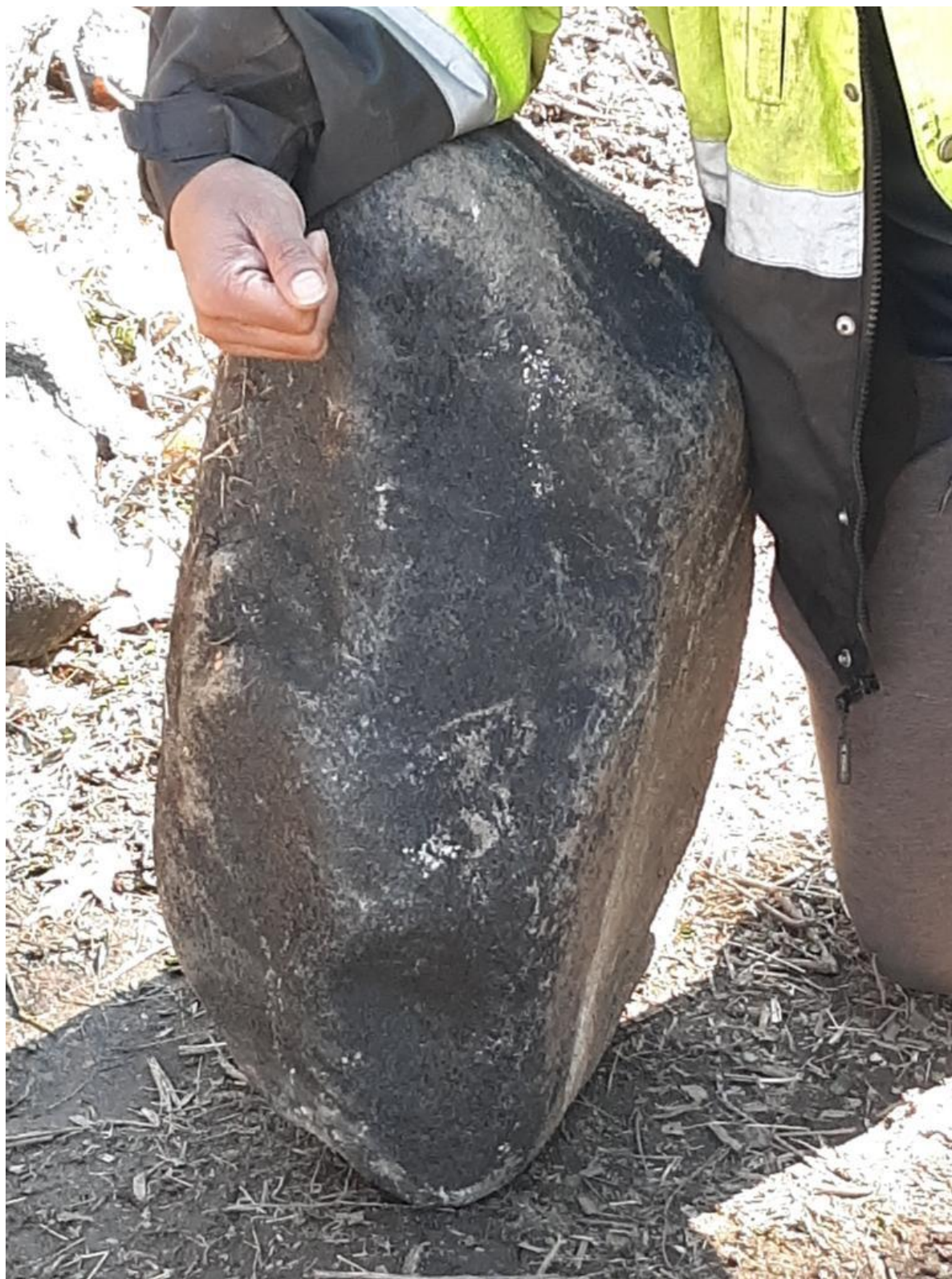
Figure 3-12: SC 977 – Heavy debris clogging sewers (Picture 3 of 3)
