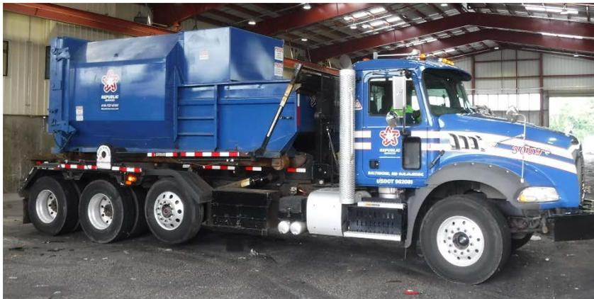
**Enclosed Compactor Container Suitable for Collecting Food Waste from Large-Capacity Customers**
